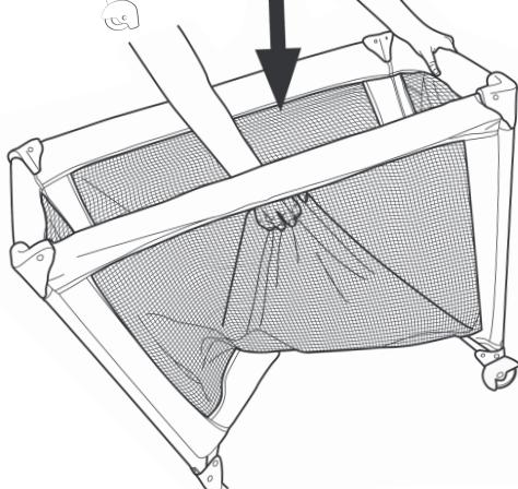
Once all 4 side rails are securely locked, hold one end of the unit up and push the center of the floor down.
